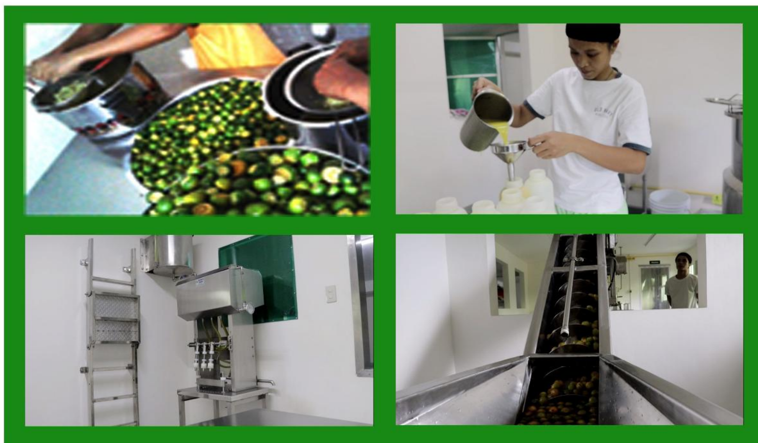
Clockwise: Manual squeezing is the RPCSE's old process of calamansi extraction. A staff is using the kitchen funnel and small stainless pitcher to put the calamansi juice into the bottle. Through the Small Enterprises Technology- Upgrading Program (SET-UP) of Department of Science and Technology (DOST), the enterprise acquired new equipment, namely, the Washing Screw Conveyor that can be used for extracting calamansi and Filler for placing the calamansi juice into the bottle.
